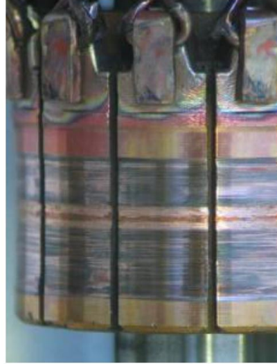
Brush / commutator after 2 x life cycle
